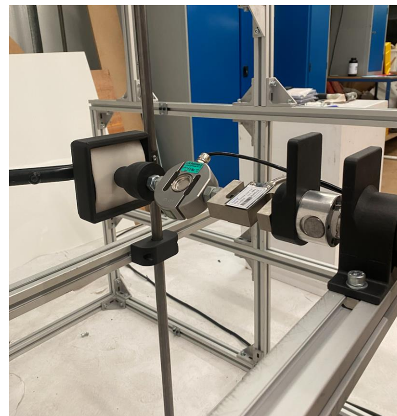
Figure 2 – Testing set-up showing the rig, container, mount and actuator
